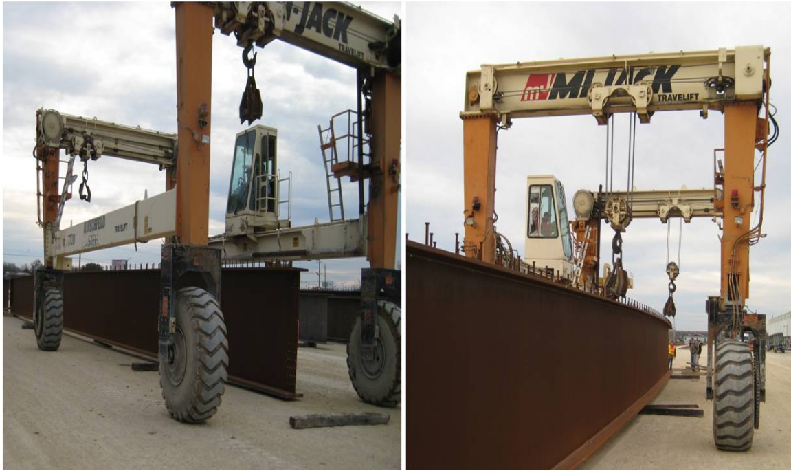
Figure 3.27 MI-JACK Travelift Provided By Hirschfeld Steel
