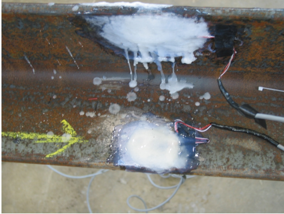
Figure 2.8 Cross Frame Gages w/ Wax and Silicone Protection
