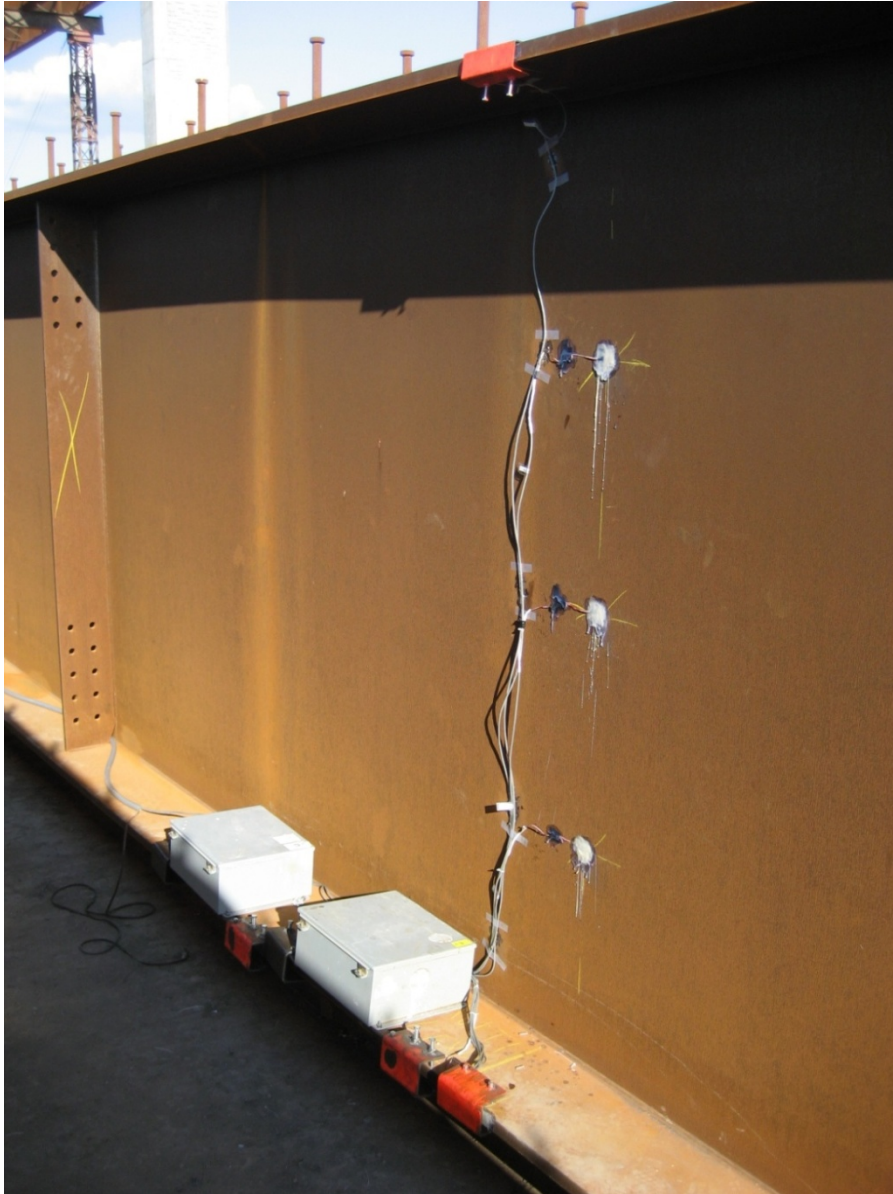
Figure 2.15 Instrumented Girder Cross Section
